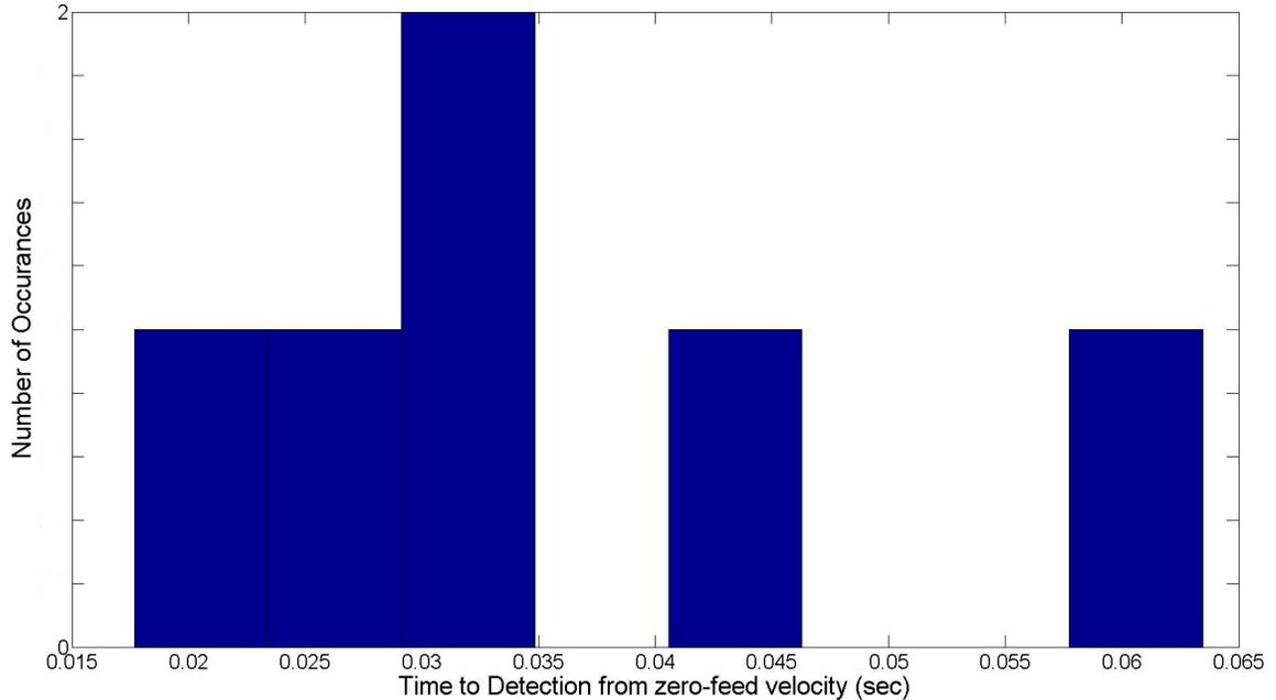
Figure 3.5. Histogram of time to detection (vibration monitoring method)
