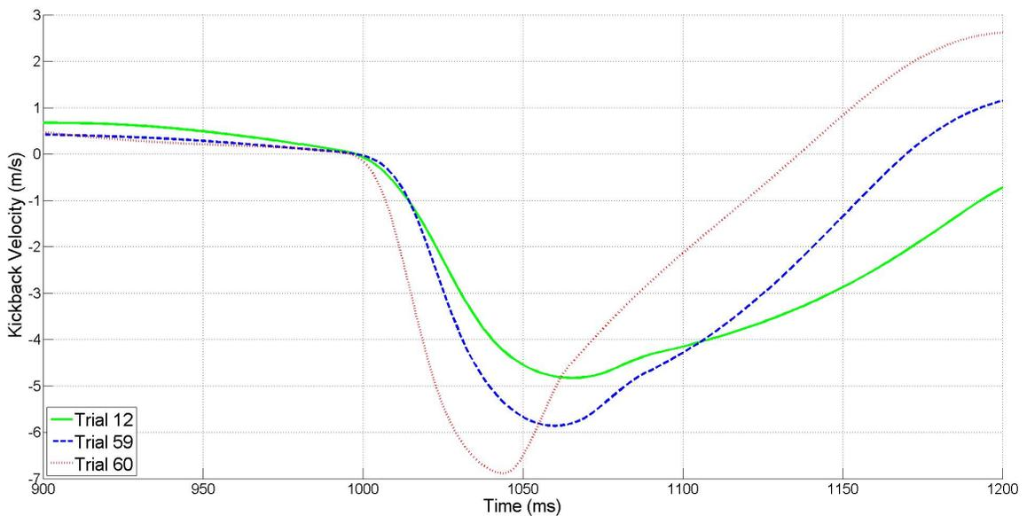
Figure 2.16. Velocity profiles of work pieces during kickback experiments
