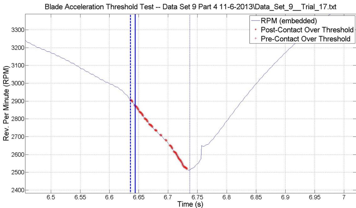
Figure 3.1. Example of detection prior to kickback start
