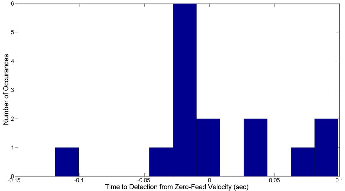
Figure 3.3. Histogram of time to detection (angular acceleration method)
