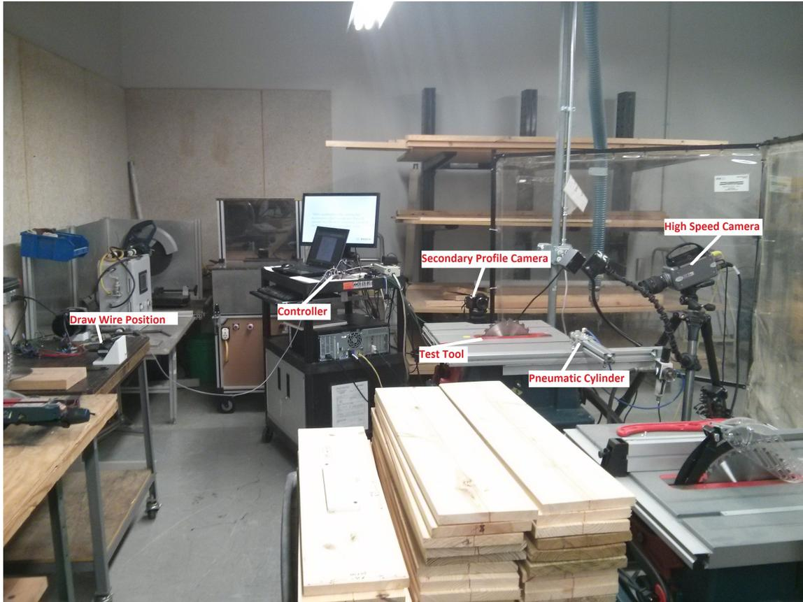
Figure 2.3. Image showing the overall experimental setup
