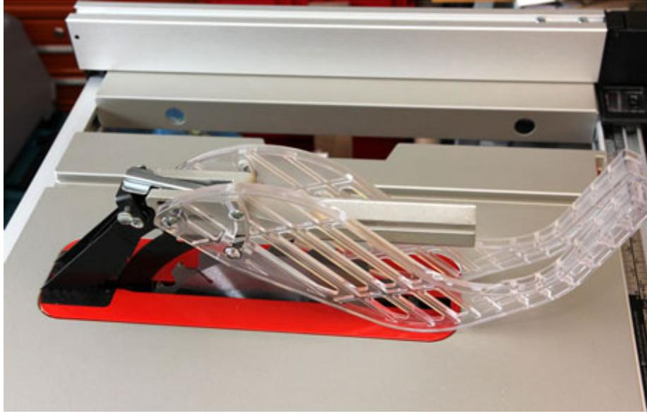
Figure 1.12. Assembly of safety devices typically standard on table saws
