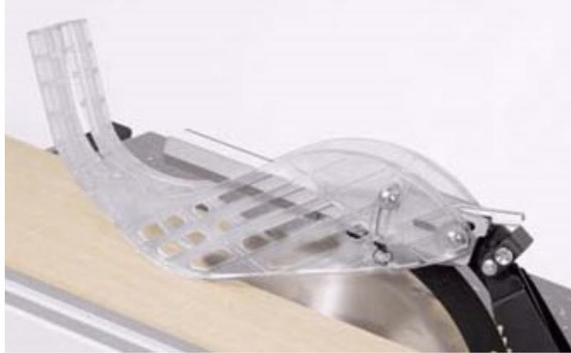
Figure 1.8. Table saw blade guard
