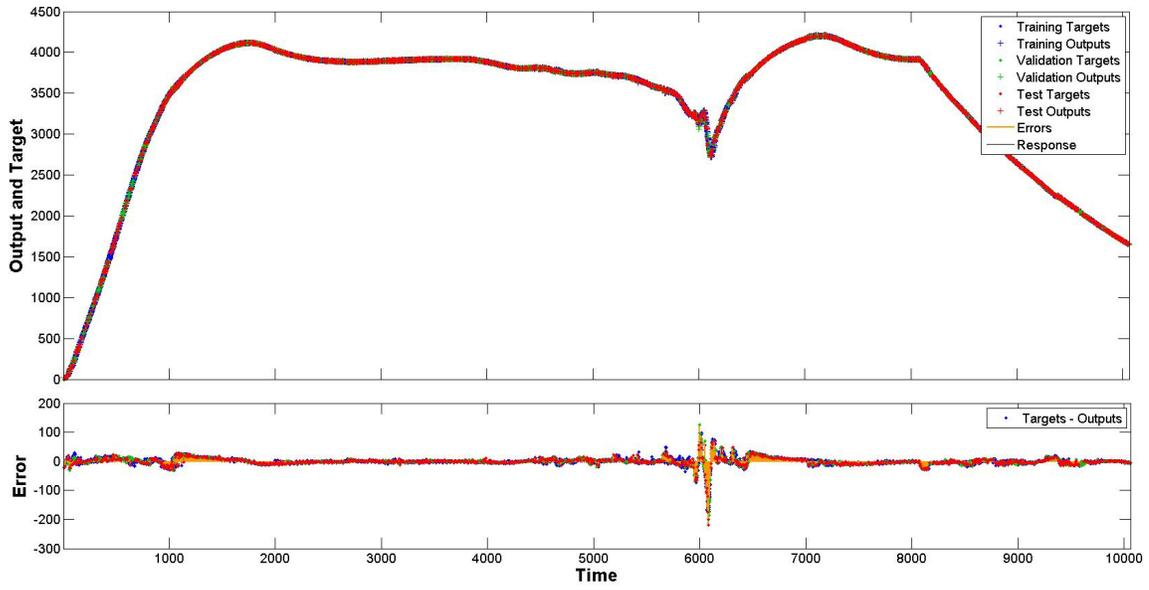
Figure B.8. Predicted time series curve of blade RPM
