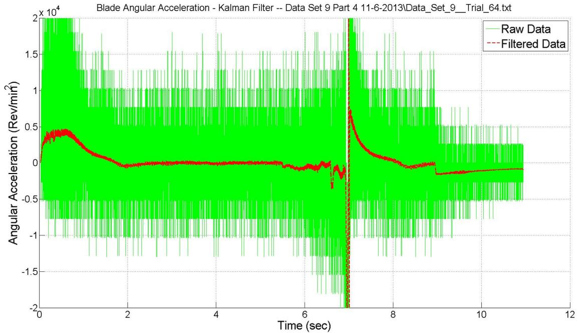
Figure 2.18. Angular acceleration derived from angular velocity
