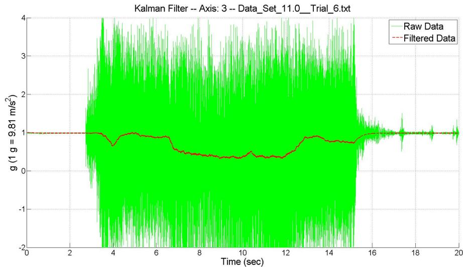
Figure 2.20. Results of filtering accelerometer data and effect of DC offset drift
