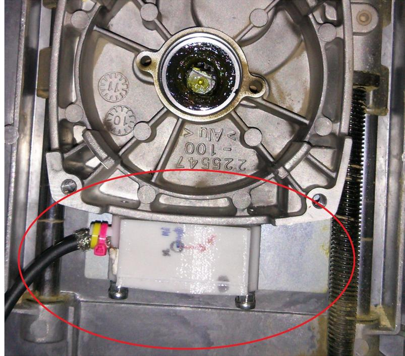
Figure 2.19. Accelerometer attachment to underside of gearbox
