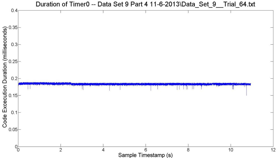
Figure 2.9. Execution duration of real-time processes per sample
