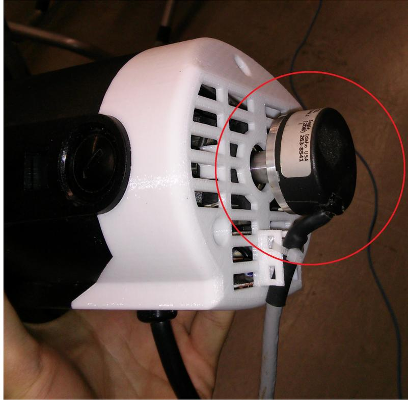
Figure 2.5. Angular velocity encoder attachment
