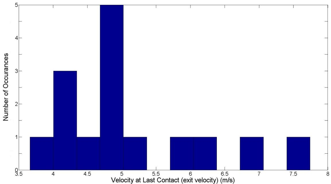
Figure 2.13. Histogram of kickback velocities at separation from saw blade
