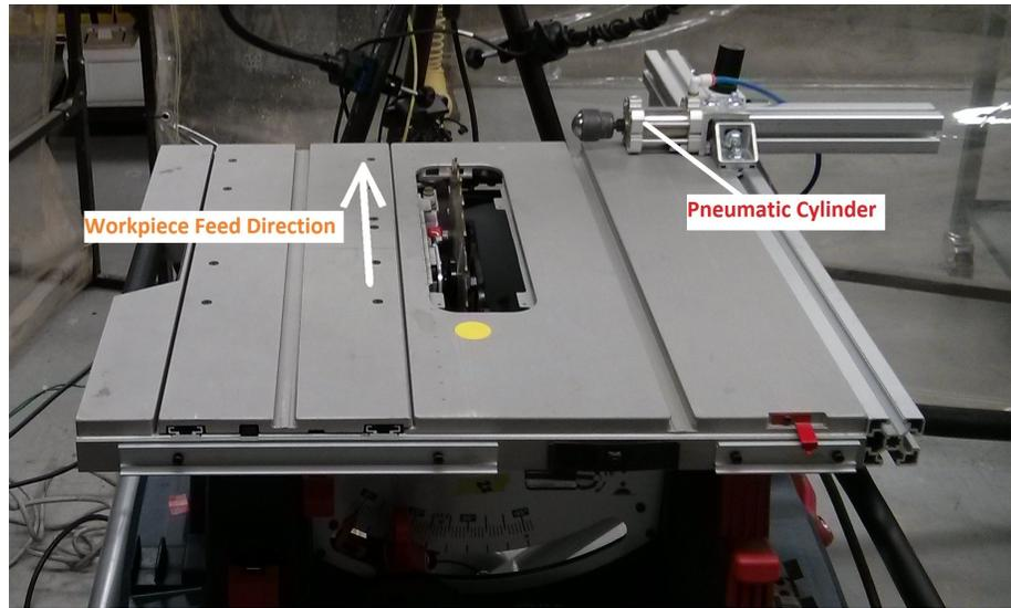
Figure 2.2. Close-up of saw table top and pneumatic cylinder
