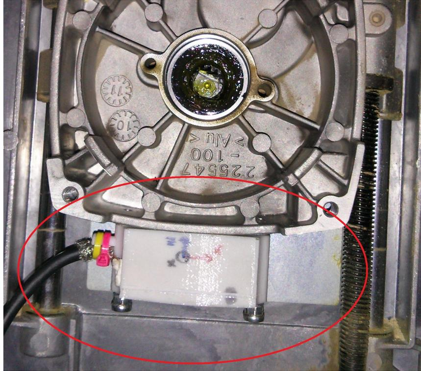
Figure 2.6. Accelerometer mounting
