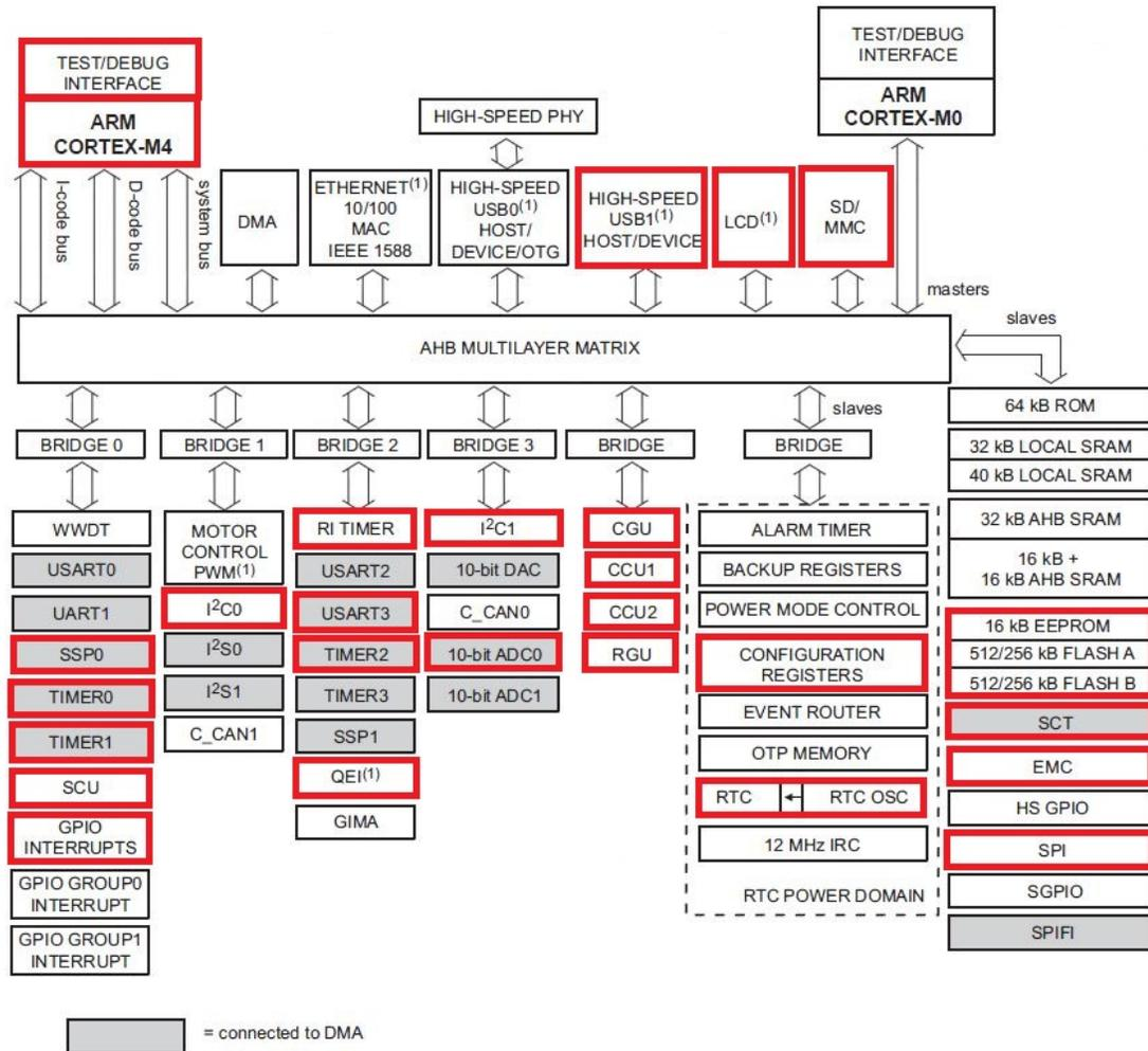
Figure 2.7. Block diagram of micro-controller (NXP LPC4357FET256)
