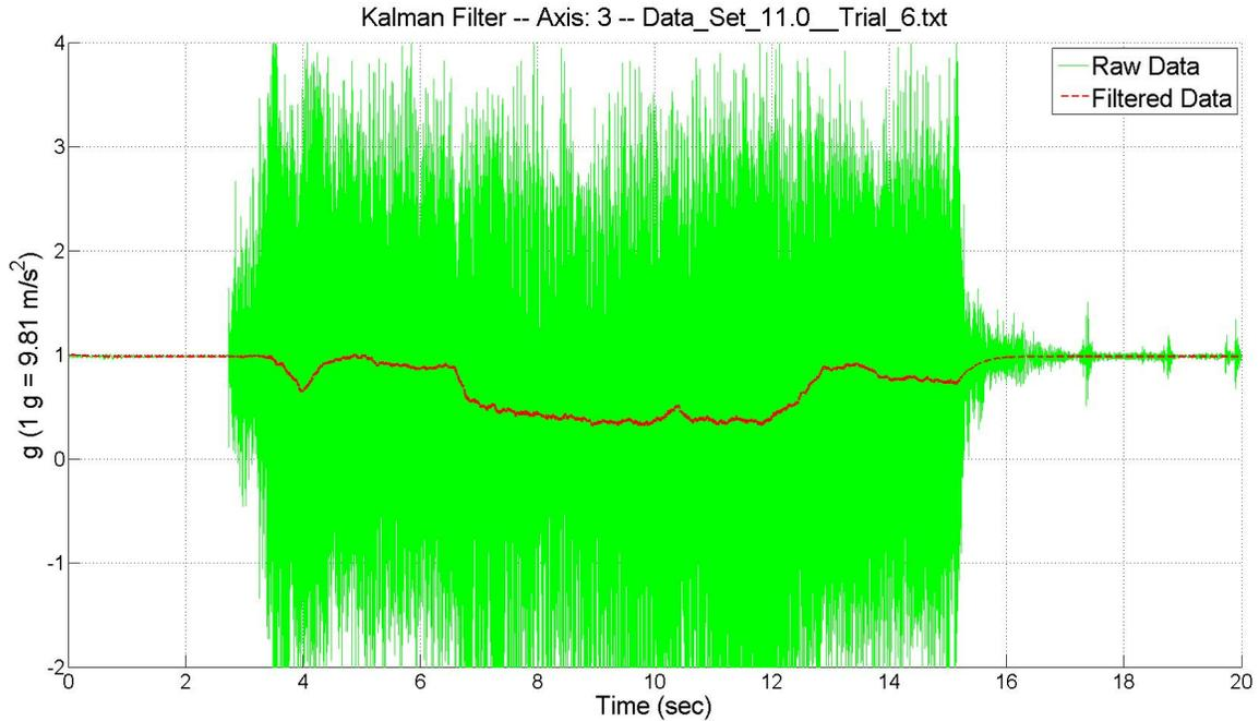
Figure 2.10. Performance of Kalman filter applied to accelerometer vibration data
