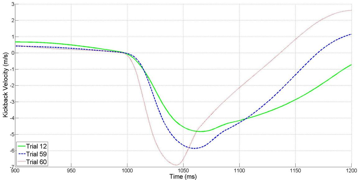
Figure 2.12. Velocity profiles of work pieces during kickback experiments
