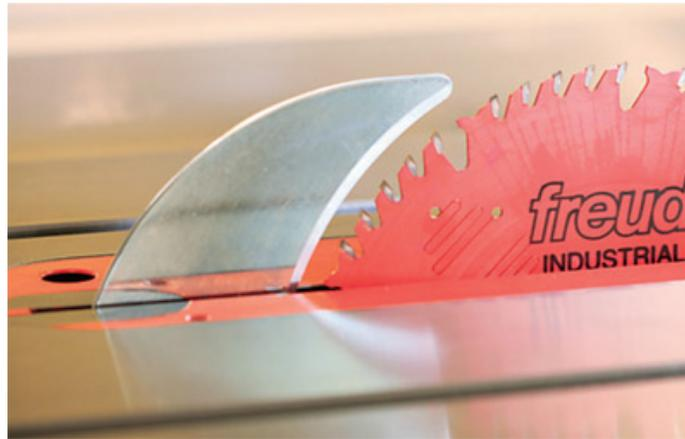
Figure 1.9. Table saw riving knife
