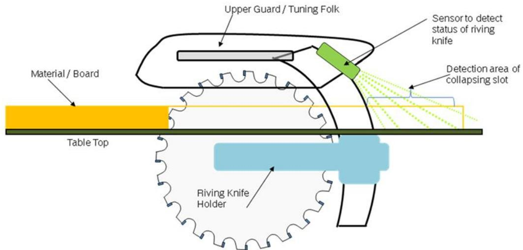
Figure B.3. Possible embodiment of Kerf sensing
