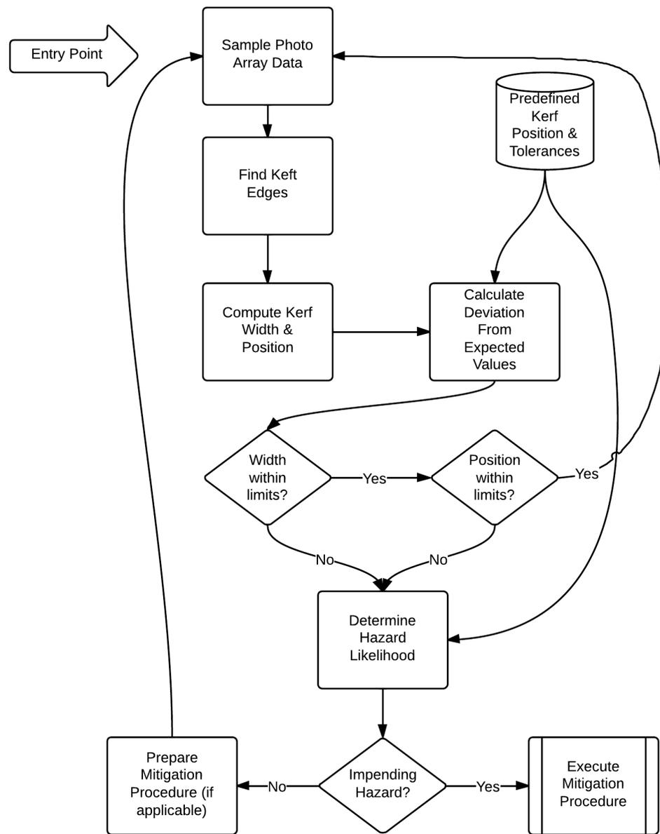
Figure B.2. Flow chart of the kerf based evaluation process)
