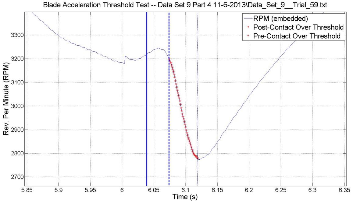
Figure 3.2. Example of detection after kickback start
