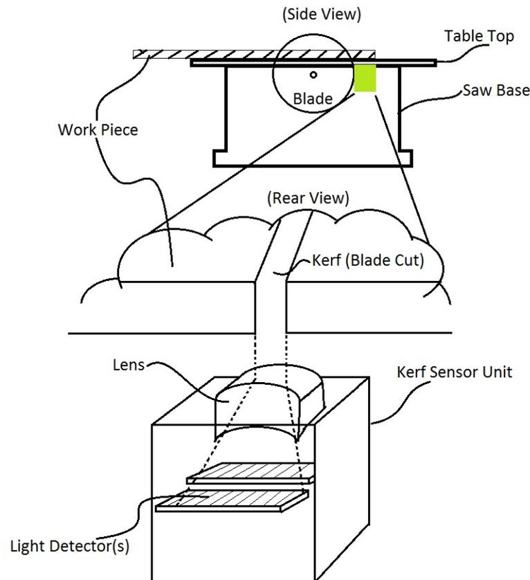
Figure B.4. Sketch of alternative cost effective sensor
