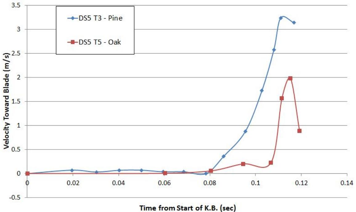
Figure 2.15. Work piece lateral velocity profile during kickback experiments
